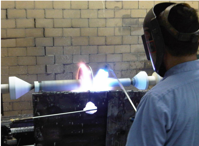
Fusing Colmonoy 52SA onto B.O.P. Ram
