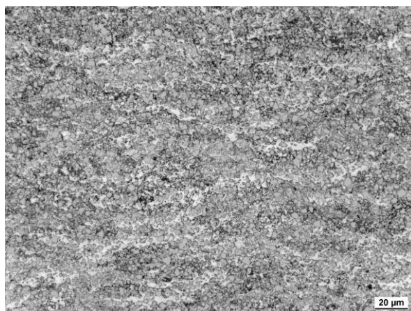
AMPERIT® 512.074: Microstructure of the coating sprayed with JP-5000
